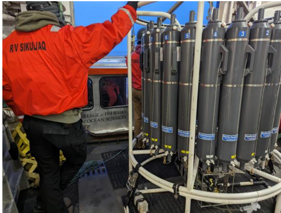
Conductivity, temperature, depth (CTD) instrumentation
