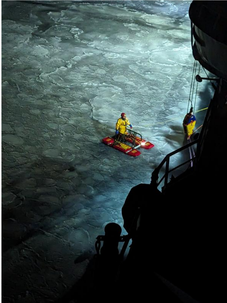
Deployment of the ARTIE (Arctic Rescue Technology for Individuals and Equipment)
